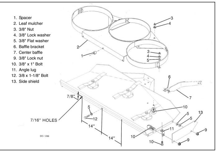
Figure 8. Optional Leaf Mulcher Installation
